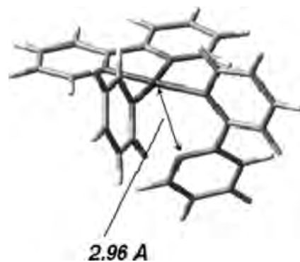
Figure 4. Proposed structure of the (\text{Pt}(\text{bpy})_2(\text{py}))^{2+} complex generated by DFT calculations. Distances for coordinating Pt–N bonds are between 2.05 and 2.10 Å, while that of Pt–N(dangling pyridine) is much longer (2.96 Å), resulting in a pseudo-five-coordinated structure.
